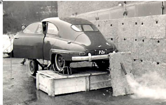
Our first assignment for Saab, a "Transfer Path analysis".
